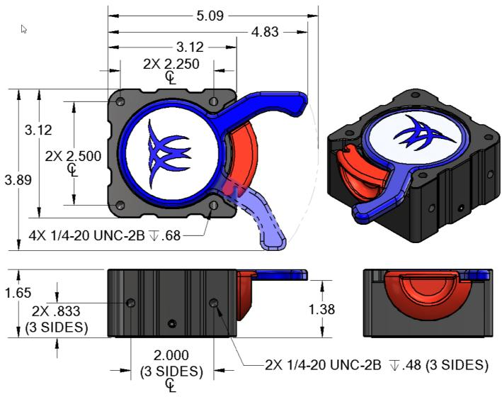
Up to 500 lbs. of holding force on 1/4" steel and thicker
